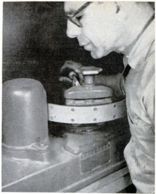
PROPER MATCHING of brake lining thickness to drum diameter generally demands grinding of the linings
