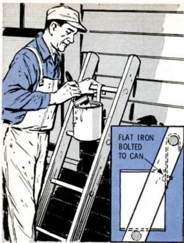
PAINT BUCKET CADDY for use when painting from a tall ladder can be made by bolting a 9-in. metal strap to an empty can and bending the end to form a hook for slipping over rung. Bucket rests on rung below
