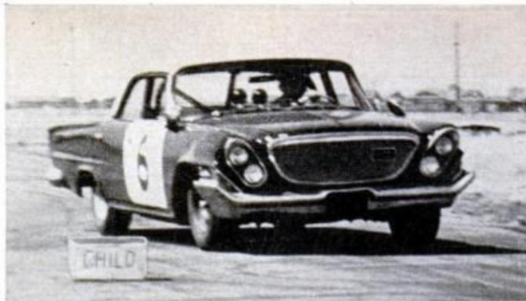
STRING attached to cardboard "child" allows box to be yanked onto roadway without warning, directly in test car's path. This time, author relies on steering instead of brakes; he swings left and misses the box easily
