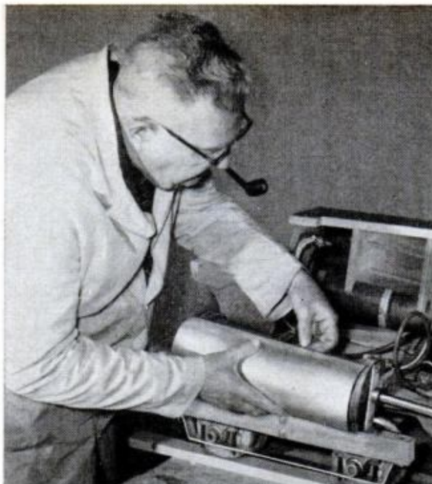
CYLINDER COVERS are light sheet metal rolled to provide friction fit over coil ends and separators. Dummy steam chests hold covers securely in place
