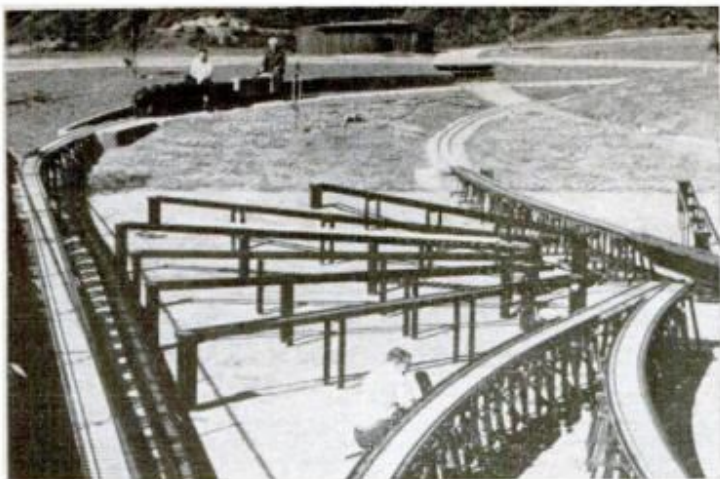
STEAMING TRACKS on Johnson's layout are used to get engines up to steam before entering main line. Entire Johnson system will be ready by 1967 season
